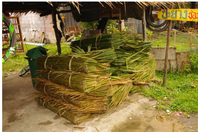
Figure 8. Roof sections made by the community in Bang Lang Da, from local Nypa palm leaves
