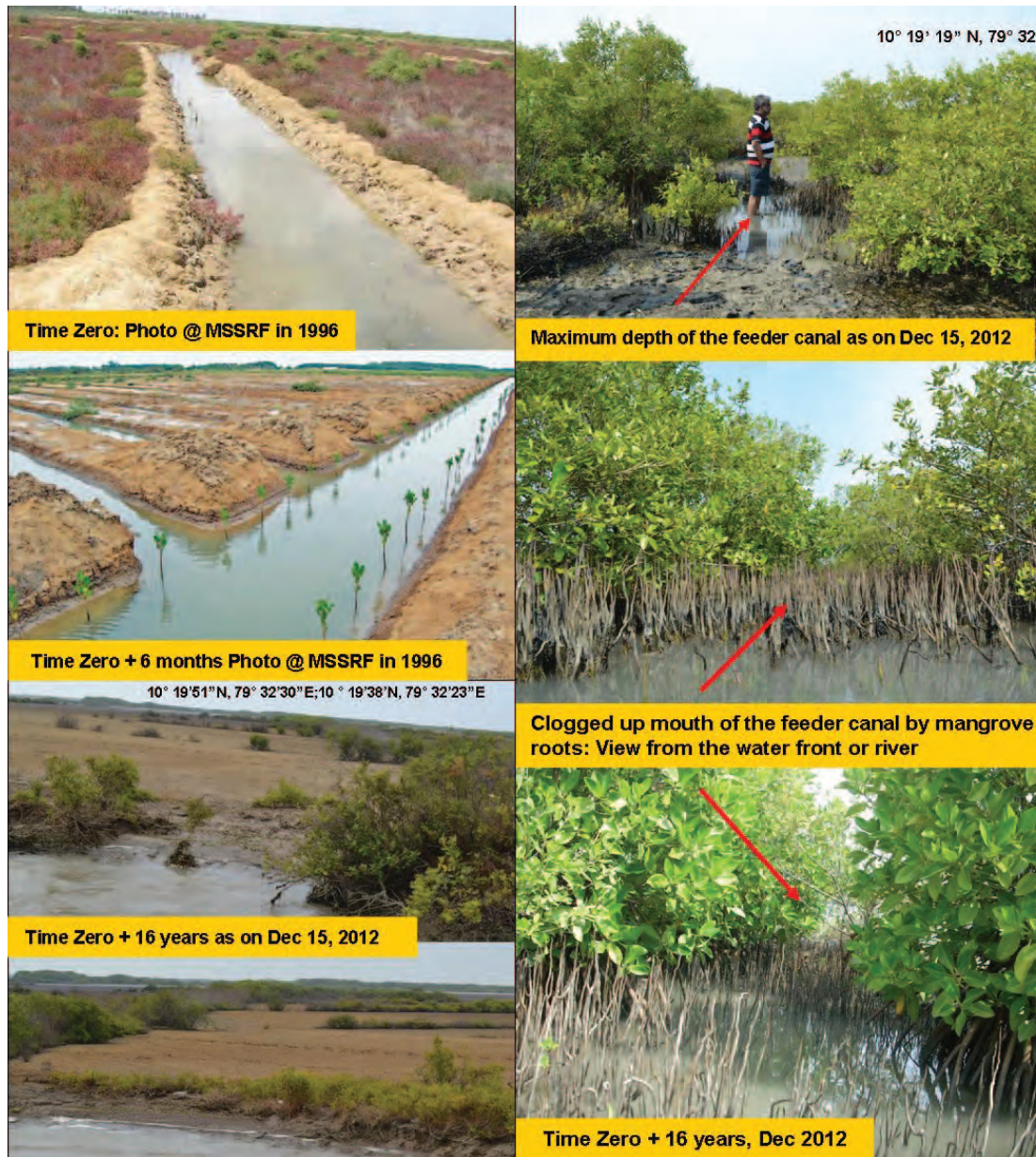
Fig 10.8 Snapshots of developments over time of fishbone canals (This page and next) Initially, canals supported adequate mangrove growth at appropriate substrate elevations. Over time, however, siltation of tidal channels caused mangrove stunting and mortality.
