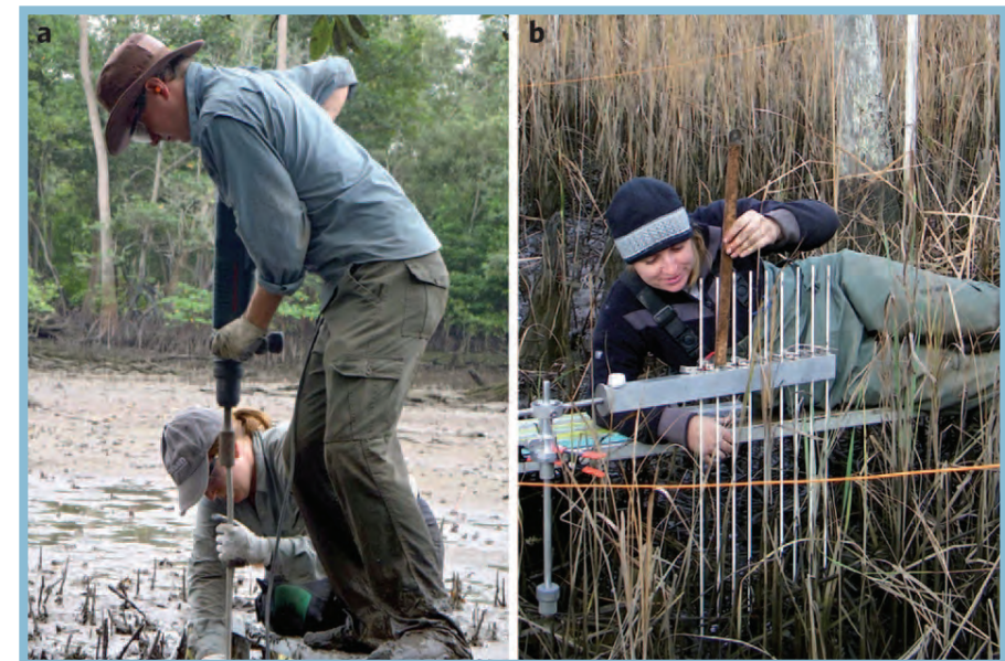
Driving an RSET rod through a mangrove soil profile (left). Measuring salt-marsh surface elevation with an RSET (right).
